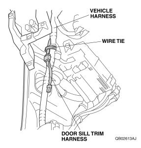
Plug the door sill trim harness 2-pin connector into the left illuminated door sill trim harness 2-pin connector.
