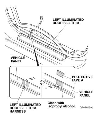
20. Install the protective clip to the protective tape A on the vehicle panel.
