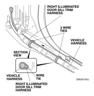
36. Secure the right illuminated door sill trim harness to the vehicle harness with two wire ties.
