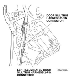
34. Bundle up the excess door sill trim harness, and secure it and 2-pin connectors to the vehicle harness with one wire tie.
